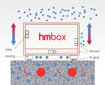
The aluminum ring of the **hm**box is fixed with fix glue to the floor.
